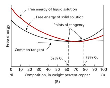
**FIG. 11.4** Free-energy-composition curves for the copper-nickel alloy system. **(A)** Freezing point of pure nickel; 1455°C **(B)** 1200°C
