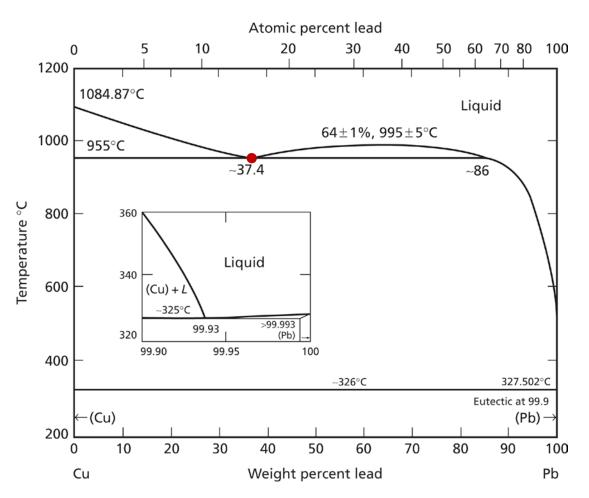
**FIG. 11.19** Copper-lead phase diagram. (From *Binary Alloy Phase Diagrams*, Massalski, T.B., Editor-in-Chief, ASM International, 1986, p. 946. Reprinted with permission of ASM International(R). All rights reserved. www.asminternational.org)
