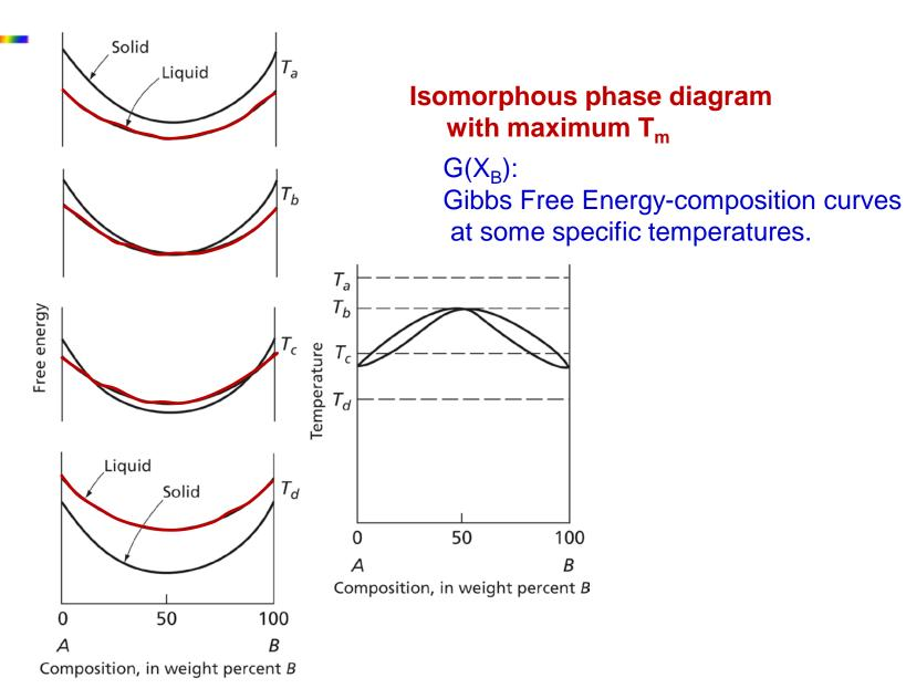
**FIG. 11.6** Relationship of the free-energy curves that lead to a maximum
