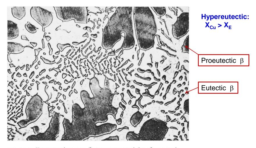
**FIG. 11.16** Hypereutectic copper-silver structure consisting of proeutectic beta (large dark areas) and eutectic.
