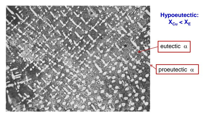
**FIG. 11.14** A hypoeutectic structure from the copper-silver phase diagram containing approximately 24 percent copper. Lighter oval regions are proeutectic alpha dendrites, while the gray background is the eutectic structure
