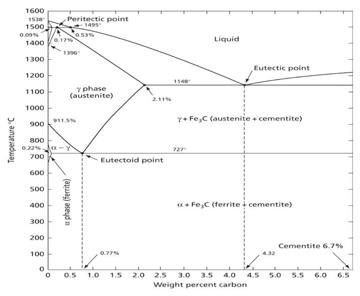
**FIG. 18.2** The Fe-Fe $_3$ C metastable phase diagram. (After Chipman, J., *Met. Trans.*, **3** 55 [1972].)
