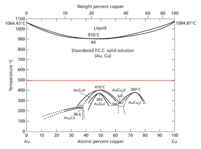
**FIG. 11.9** Copper-gold phase diagram. (From *Bulletin of Alloy Phase Diagrams*, Vol. 8, No. 5, by Okamoto, H., Chakrabarti, D. J., Laughlin, D. E., and Massalski, T. B., 1987, p. 454. Reprinted with permission of ASM International (R). All rights reserved www.asminternational.org)
