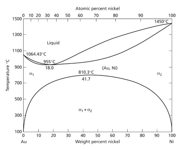
**FIG. 11.7** Gold-nickel phase diagram. (From *Binary Alloy Phase Diagrams*, Massalski, T.B., Editor-in-Chief, ASM International, 1986, p. 289. Reprinted with permission of ASM International(R). All rights reserved. www.asminternational.org)
