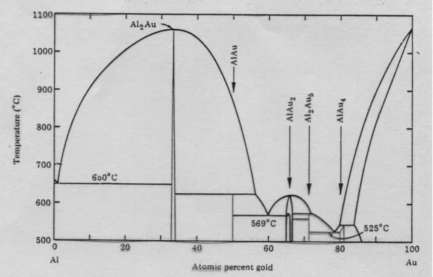
FIGURE 11.14 Phase diagram of the Au-Al system. [Adapted from the Bull. Alloy Phase Diagrams 8(1), 71 (1987).]
