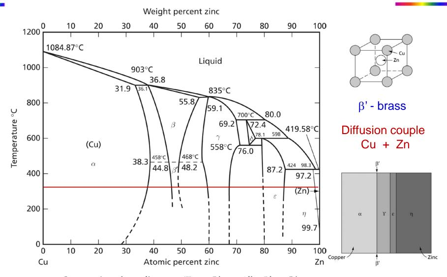
**FIG. 11.23** Copper-zinc phase diagram. (From *Binary Alloy Phase Diagrams*, Massalski, T.B., Editor-in-Chief, ASM International, 1986, p. 981. Reprinted with permission of ASM International(R). All rights reserved. www.asminternational.org)
