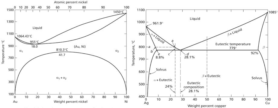
**FIG. 11.7** Gold-nickel phase diagram. (From *Binary Alloy Phase Diagrams*, Massalski, T.B., Editor-in-Chief, ASM International, 1986, p. 289. Reprinted with permission of ASM International(R). All rights reserved. www.asminternational.org)
