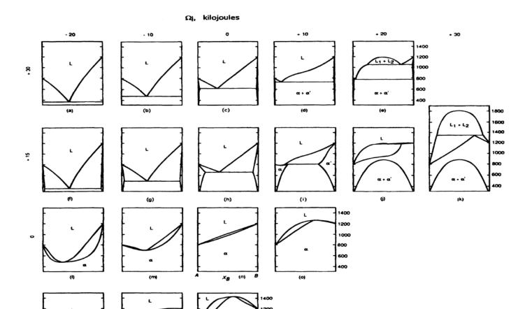
Figure 10.23 Topological changes in the phase diagram for a system A–B with regular solid and liquid solutions, brought about by systematic changes in the values of  $\Omega_s$  and  $\Omega_l$ . The melting temperatures of A and B are, respectively, 800 and 1200 K, and the molar entropies of melting of both components are 10 J/K. (From A. D. Pelton and W. T. Thompson, *Prog. Solid State Chem.* (1975), vol. 10, part 3, p. 119).
