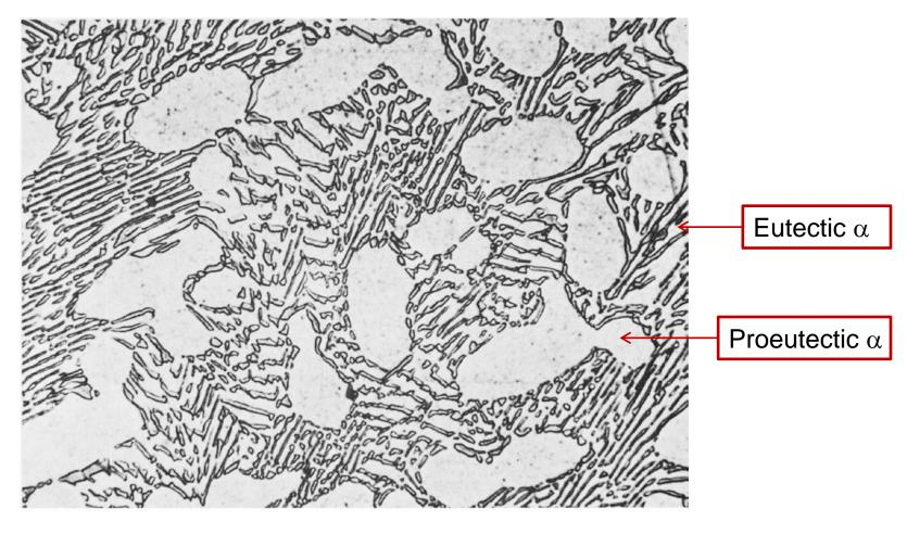
**FIG. 11.15** The microstructure of Fig. 11.14 shown at a greater magnification. (White matrix is the alpha or silver-rich phase. Dark small platelets are the beta or copper-rich phase. The eutectic structure is thus composed of beta platelets in an alpha matrix.)
