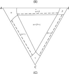
**FIG. 11.27** Three isothermal sections for the ternary diagram shown in Fig. 11.26. A few of the tie lines are shown by the dotted lines. **(A)** At a temperature below *A-B* eutectic temperature but above eutectic temperatures of the ternary, *A-C* and *B-C*; **(B)** at a temperature below the three binary eutectics but above the ternary eutectic, and **(C)** at a temperature below the ternary eutectic temperature
